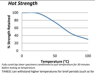
paint baking and wave soldering processes) providing the joint is not unduly stressed. The minimum temperature the cured adhesive can be exposed to is -55°C depending on the materials being bonded.
