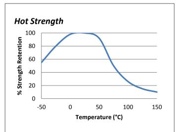
"Hot strength" shear strength tests performed on mild steel. 24hr cure at room temperature and conditioned to pull temperature for 30 minutes before testing.
