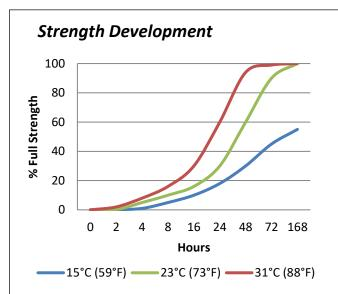
Graph shows typical strength development of bonded components. An increase of  $8^{\circ}$ C (46°F) in temperature will halve the cure time. Lower temperatures will result in a slower cure time.
