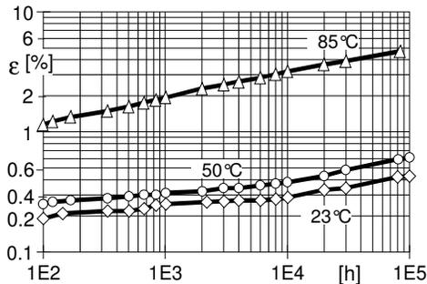
Fig.7.5: **Elongation (ε) in function of time at 23, 50 and 85°C**
