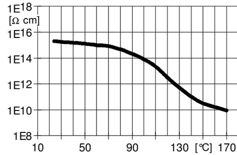
Fig.6.2: **Volume resistivity ( $\rho$ ) as a function of temperature**
