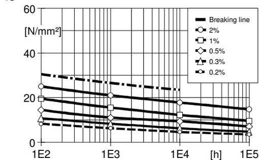
Fig.7.8: **Creep diagram at 85°C**
