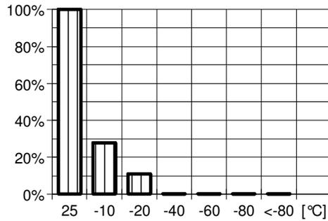
Fig.8.1: **Crack resistance / Temperature shock test**
