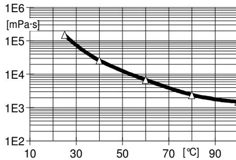
Fig.4.2: **Initial viscosity as a function of temperature**
