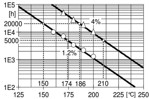
Fig.7.2: **TI 150 / 174** (weight loss 1.2%)
