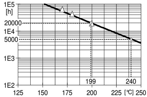
Fig.7.4: **TI 199 / 240** (flexural strength)
