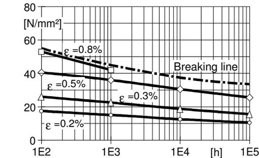
Fig.7.6: **Creep diagram at 23°C**
