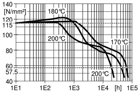
Fig.7.3: **Loss of flexural strength** (limit: 50%)
