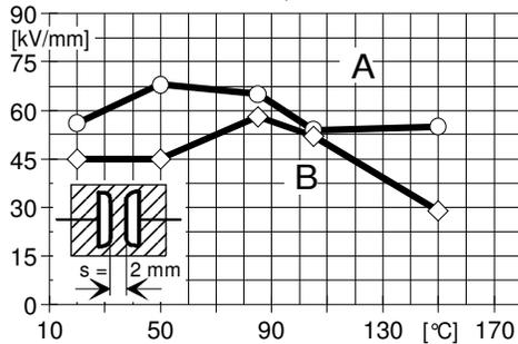
Fig.6.3: **Breakdown field strength ( $E_d$ ) as a function of temperature**
