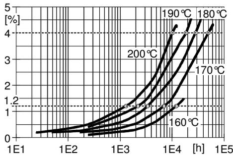
Fig.7.1: **Weight loss** (specimen: 50x50x3 mm)
