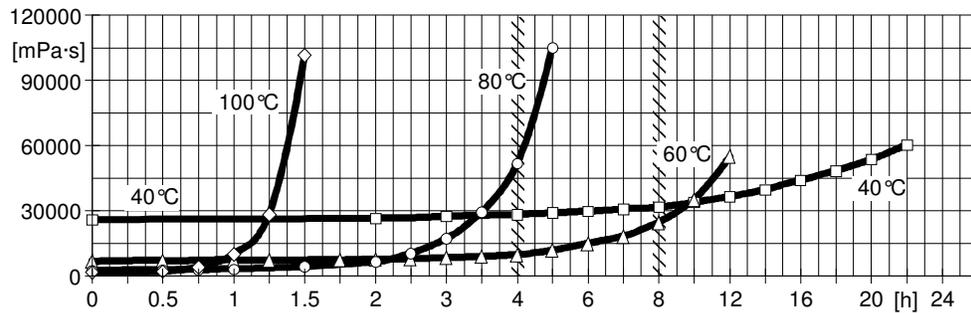
Fig.4.1: **Viscosity increase at 40, 60, 80 and 100 °C** (measurements with Rheomat 115)
