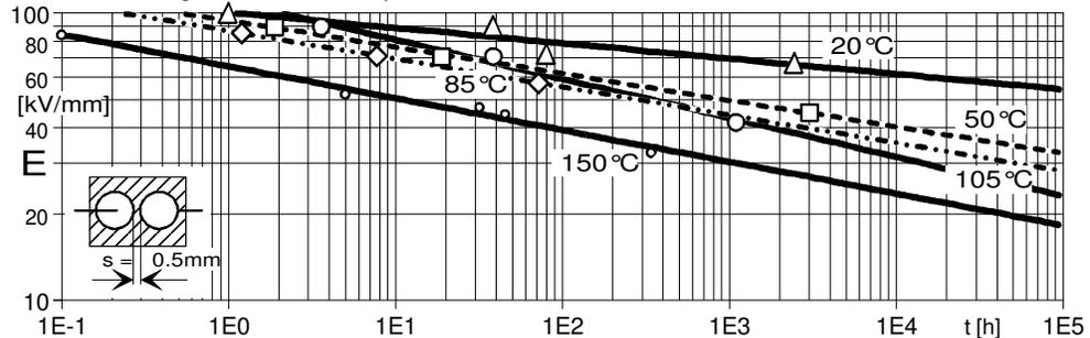
Fig.6.4: **Life time curves of the electric field stress ( $E$ ) at 20, 50, 85, 105 and 150 °C**
