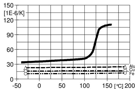
Fig.5.2: **Coefficient of linear thermal expansion ( $\alpha$ ) in  $f(T)$**  (ISO 11359-2, reference temperature: 23°C)
