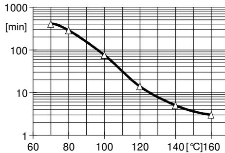
Fig.4.4: **Gellime as a function of temperature**
