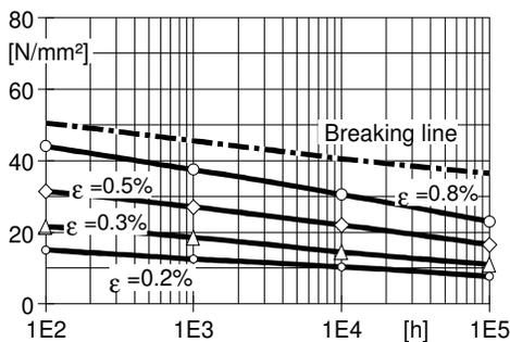
Fig.7.7: **Creep diagram at 50°C**
