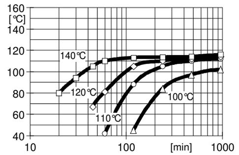
Fig.4.5: **Glass transition temperature as a function of cure time**
