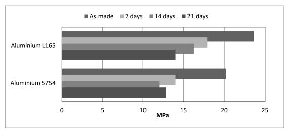
Lap shear strength versus immersion in various media (ISO4587) (typical average values)
