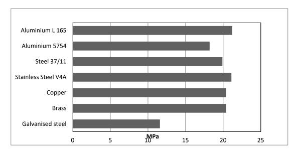
Average lap shear strengths of typical metal-to-metal joints (ISO 4587) (typical average values)
