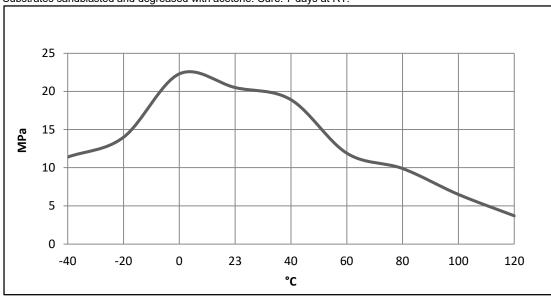
Lap shear strength versus temperature (ISO 4587) (typical average values) Substrates sandblasted and degreased with acetone. Cure: 7 days at RT.
