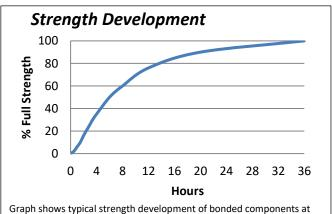
Graph shows typical strength development of bonded components at 23°C. Curing at higher or lower temperatures may affect cure speed.
