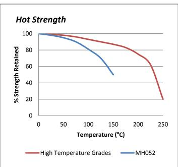
"Hot strength" Breakaway strength on M10 Zinc plated bolts according to ISO 10964. Cured at 23  $^{\circ}$ C for 24 hours then conditioned for 30 minutes at testing temperature.
