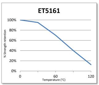
ET5161 can withstand higher temperatures for brief periods (such as for paint baking and wave soldering processes) providing the joint is not unduly stressed. The minimum temperature the cured adhesive can be exposed to is -55°C (-67°F) depending on the materials being bonded.
