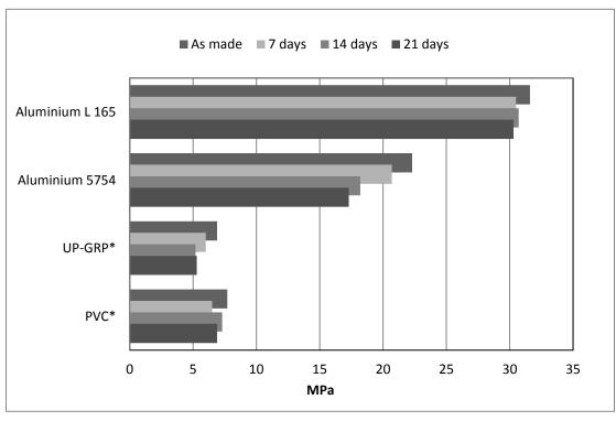
(\*): UP-GRP, PVC, substrate failure
