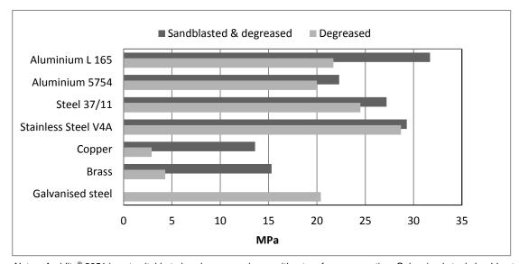
Notes: Araldite<sup>®</sup> 2051 is not suitable to bond copper or brass without surface preparation. Galvanised steel should not be abraded or sandblasted, better results are obtained with only degreasing.
