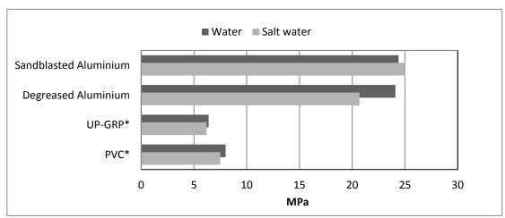
(\*): UP-GRP, PVC, substrate failures observed.
